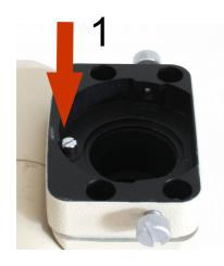
Remove the old adapter solution. Only the photo tube should remain. There is a small set screw on the photo tube, which is not needed with the new LM adapter solution. If the TUST42C\_SZ can't be fitted properly because of this set screw, we recommend to simply remove the screw.
