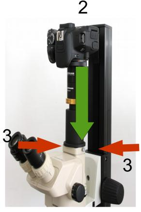
Remove the set screw (image 1). Now loosen the two knurled screws (3) and plug the TUST42C\_SZ in to the photo tube (2). Then fix the C-Mount Port 1x by tightening the two knurled screws. The TUST42C\_SZ should be mounted securely.
