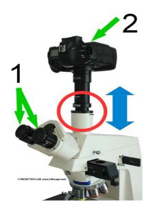
Than you should adjust parfocality (sharp image on observation tube and photo at the same time).
