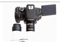
Next, fit the LM digital SLR universal adapter for 23.2 mm tubes into the TUST30 tube adapter and secure it in place by tightening the three Allen head screws.
