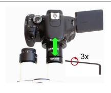
To achieve optimum focus, you have the possibility (as described above) of adjusting the distance between tube adapter and LM digital adapter using an Allen key.
