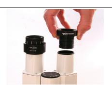
Check how much extra space there is around the tube adapter without O-rings, and then use the larger or the smaller rings accordingly. You can also use a combination of larger and smaller O-rings.
