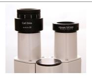
The tube adapter should fit into the eyepiece tube without being forced, and should not wobble when inserted.
