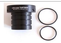
Depending on the brand and model of the microscope, the interior diameter of the eyepiece tube might differ by a few tenths of a millimetre from the measurement required. For this reason, the tube adapter [TUST30W and TUST30S] comes with several different O-rings included. This allows the user to achieve an exact fit.
