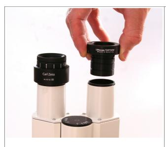
Check how much extra space ther is around the tube adapter without O-rings, and then use the larger or the smaller rings accordingly. You can also use a combination of larger and smaller O-rings.
