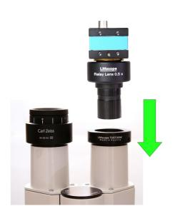
You can now connect the entire unit (LM Relay Lens Adapter and camera) into the eyepiece tube of your microscope.
