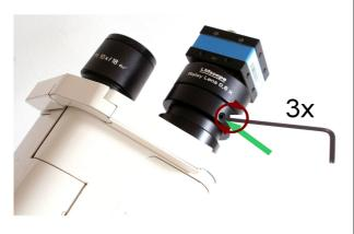
Using an Allen key, you can now fix the LM Relay Lens Adapter.
