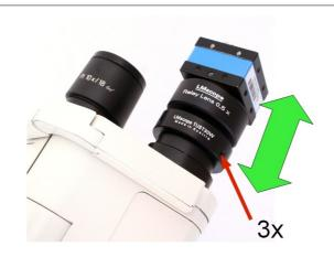
2) Focusadjustment: To achieve optimum focus, you have the possibility (as described above) of adjusting the distance between C-mount extension and LM digital adapter using an Allen key.
