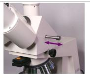
If your microscope does not have a beam splitter (e.g. 60/40), remember to adjust the deflecting prism so that light can enter into the phototube
