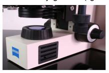
Whenever possible, bright microscope illumination, halogen illumination, LED or a flash unit designed for short flash durations is recommended. If needed, you can insert a daylight filter (light blue) into the illumination beam path or use your camera's controls to adjust the white balance.
