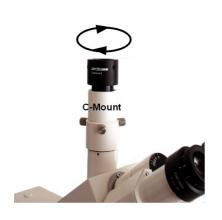
Now screw the C-mount extension onto the phototube of your microscope in a clockwise direction.
