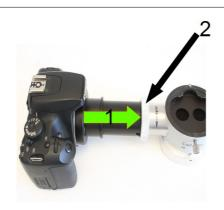
Plug the entire unit (camera/adapter) into the beam splitter's tube. Pay attention to the positioning groove (see no 1 in the picture)!
