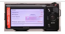
With some cameras, a shutter release is only possible with the lens being in place. If this is the case with your camera, select the "release without lens" point in the set-up menu (wording varies from manufacturer to manufacturer).
