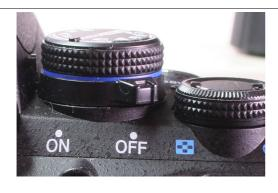
Switch the camera on and, if possible, use the automatic control program. If that is not possible, use the "automatic aperture control" setting. If these two options do not work, you can also work in "M" (manual) mode. We recommend that you extend the power saving mode on your camera, otherwise the camera will constantly switch itself off.
