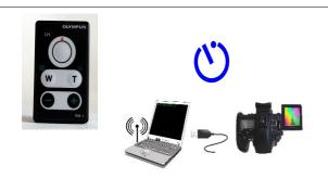
Blurred images are mostly caused by releasing the shutter manually. This leads to vibrations, which are picked up as motion blurs in the images. To avoid motion blurs, we recommend that you use a remote control release. Otherwise it is also possible to use the digital camera's self-timer function. Using a remote control software is also ideal (controlled from the PC); unfortunately, this is not supported by every camera.
