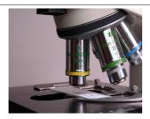
Now swivel into the lowest magnification and visually focus the image by means of the microscope focusing mechanism. Plan achromatic, plan fluor or plan apochromatic microscope lenses are optimal for perfect micro images.
