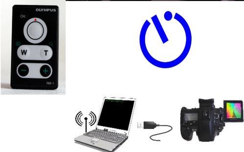
Blurred images are mostly caused by releasing the shutter manually. This leads to vibrations, which are picked up as motion blurs in the images. To avoid motion blurs, we recommend that you use a remote control release. Otherwise it is also possible to use the digital camera’s self-timer function. Using a remote control system is also ideal (controlled from the PC); unfortunately, this is not supported by every camera.
