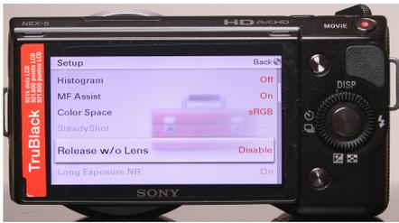
With some cameras, a shutter release is only possible with the lens being in place. If this is the case with your camera, select the “release without lens” point in the setup menu (wording varies from manufacturer to manufacturer).
