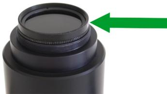
(2) Then, screw the optical filter onto the filter holder.
