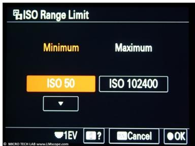
In conditions with homogeneous illumination and high light intensity, the **best results are obtained at low ISO sensor settings (50 to 200)**.
