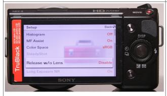
With some cameras, a shutter release is only possible with the lens being in place. If this is the case with your camera, select the "release without lens" point in the setup menu (wording varies depending on manufacturer).
