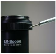
If needed, the camera can be turned to another position with the three small screws of the T2-ring.
