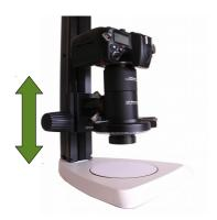
Approach the lens' front to the specimen by considering the working distance.
