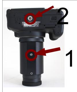
LM Photomicroscope can also be used with stands from other manufacturers with the help of the tripod socket.
