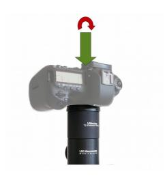
Now attach the microscope to your camera using the bayonet mount. Make sure that the tip of the bayonet thread is exactly on the tip of the camera thread before turning clockwise. With some camera models it is necessary to hold down the button for releasing the camera thread.
