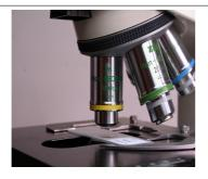
Now swivel in the 10x microscope lens and visually focus the image by means of the microscope focusing mechanism. Plan achromatic, plan fluor or plan apochromatic microscope lenses are optimal for perfect micro images.
