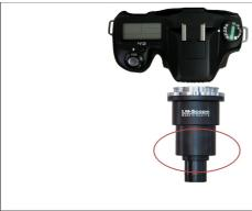
Attach the LM digital adapter to your camera using the bayonet mount. Make sure that the tip of the bayonet thread is exactly on the tip of the camera thread before turning clockwise until it locks into place. If necessary, hold down the button for releasing the camera thread.
