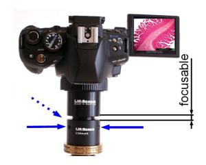
To achieve optimum focus, you have the possibility (as described above) of adjusting the distance between C-mount extension and LM digital adapter using an Allen key.
