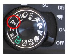
If possible, use the automatic control program. If that is not possible, use the "Aperture Priority (Av/AE)" setting. If these two options do not work, you can also work in "M" (manual) mode. We recommend that you extend the power saving mode of your camera, otherwise the camera will constantly switch itself off.
