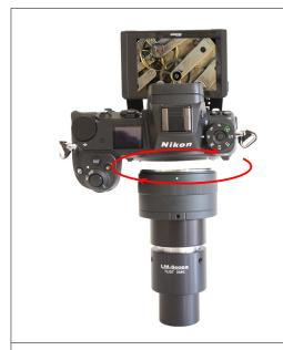
Attach the LM digital adapter to your camera using the bayonet mount. Make sure that the tip of the bayonet thread is exactly on the tip of the camera thread before turning clockwise until it locks into place. If necessary, hold down the button for releasing the camera thread.
