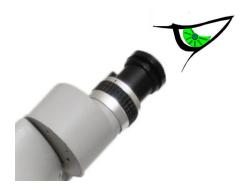
Focus adjustments to achieve parfocality can be made with the adapter solution.
