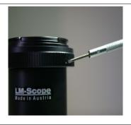
If the camera is not aligned right, you can loosen the three small screws of the T2 ring to turn it to another position.
