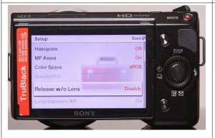
With some cameras, a shutter release is only possible with the lens being in place. If this is the case with your camera, select the "release without lens" point in the setup menu (wording varies from manufacturer to manufacturer).
