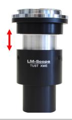
Carefully move the upper part of the adapter up or down while checking the live image on the camera screen. By adjusting the height of the camera, you can fine tune the focus.
