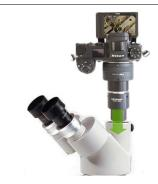
Turn on the camera. Checking the live image on the camera screen or on the monitor connected to the camera, you can now adjust the tube height to bring the image into focus.
