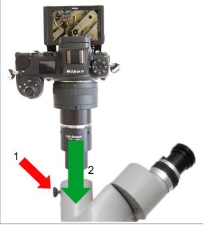
If another adapter is installed on the microscope, remove it completely so that only the phototube (36 mm internal diameter) remains.
