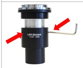
If more adjustment is necessary, the adapter can also be used to adjust the height of the camera to suit the focus of the eyepieces. For this, loosen the three Allen screws at the level of the "LM-Scope" label.
